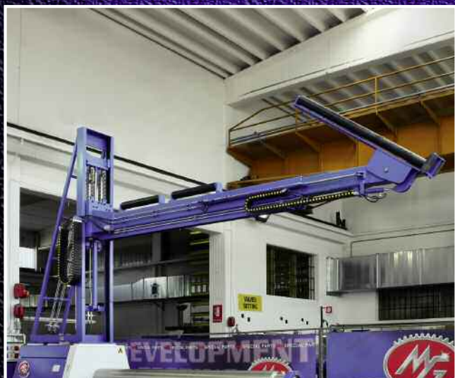
• Supporto verticale per lavorazioni coniche • Vertical support for conical bending • Support vertical pour le traitement conique • Soporte vertical para mecanizado cónico
