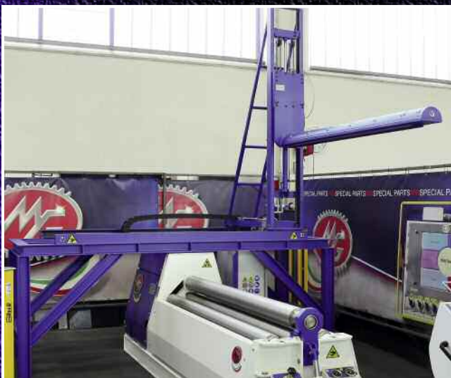
• Supporto verticale traslabile • Vertical movable support • Support mobile vertical • Soporte móvil vertical
